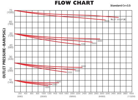
FLOW RATE - SCFM (LPM) Air (\*1 LPM=28.3 SCFM\*) FLOW RATE L/Min AIR
